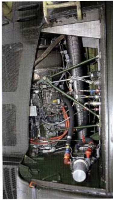
Rugged and reliable Lycoming (Honeywell) T53-L-13B producing 1400shp
