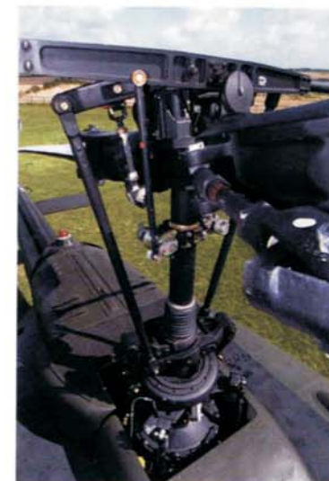
Close-up of the two-blade rotor system that gives the 'Huey' its signature noise.
